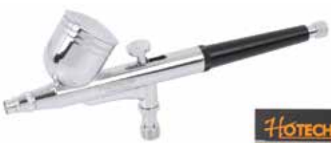
Air Brush Kit - Gravity Feed Type - 0.3mm Nozzle - 15-50psi
