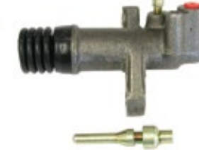
22.22mm Clutch Slave Cylinder Isuzu TFR CS14
