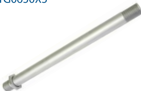
Steering Tube Models: 75-90Hp Length:310mm OD:22mm Id:16mm YG0650X5
